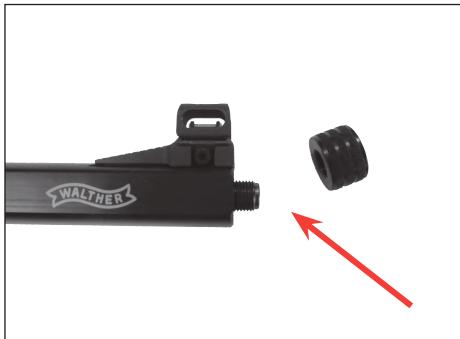
To attach the silencer, first remove the barrel nut.
