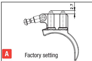
When the rifle comes from the factory, the trigger is preset as shown in Figure A. Adjust only one screw at a time, and test to see the effect on the rifle's operation. Turn the screw in to reduce the trigger weight and trigger travel. Turn the screw out to increase the trigger weight and trigger travel.
