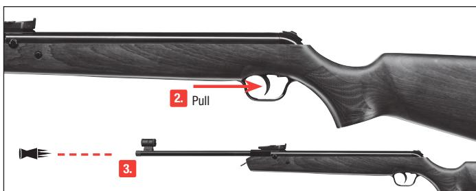
Never pull the trigger when the barrel is broken open (exception - decocking, see above).
