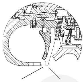
Turning screw 1 anticlockwise reduces the trigger pull force
