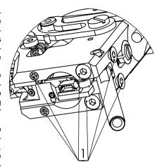
plug the electronics connector. The plug connector on the housing need not be disconnected.
