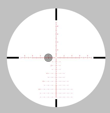
2 mil wind correction for 15 mph wind from right to left at 500 yards. Elevation turret has been dialed up to compensate bullet drop, just simply use center horizontal cross line to holdover for wind correction
