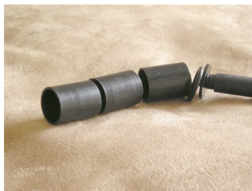
Picture 2: The components are assembled in the sequence shown above, open end in first. When all 3 components are inserted, the O ring is fitted and the disk last. The holes in all sections are threaded to allow the tool provided to screw in for ease of removal. The fit of the components should not be tight on the outside. Keep components clean. A small amount of O ring compression is felt on final tightening .
