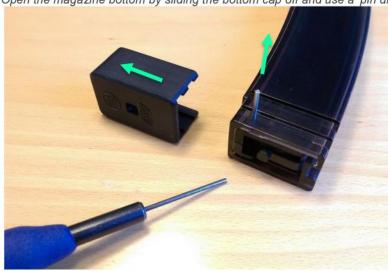
NOTE the magazine inner part is no longer locked and can be pushed out which is not necessary to do in order for you to mount your design – If you do anyway – beware of the springs!
