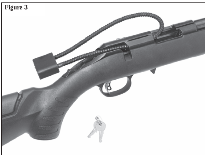
Correct Installation of Lock For RUGER AMERICAN RIMFIRE®
