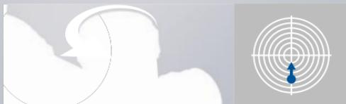
To move the central shot point **up** – turn the vertical adjustment knob toward the 'UP' arrow.
