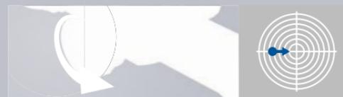
To move the point of impact **rightward** – turn the horizontal adjustment knob toward the 'R' arrow.
