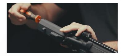
To adjust your FPS, remove your stock assembly and battery storage cap. Once these are removed, use a Philips screw driver to remove the screw. Once this is removed use the included Allen key and insert it through the hole the Philips screw came out of and twist for more or less FPS.
