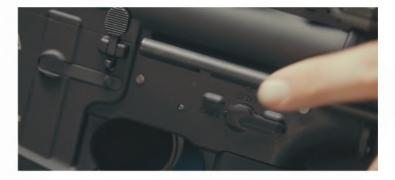
The selector which can be found on either side of the gun had 3 modes, safe, semi, and full auto. On safe, an internal mechanism will prevent the gun from firing. On semi, only one bb's will be shot out per trigger pull. On full auto, bb's will continue to be shot until the trigger is released. Once done firing always put the gun on safe.
