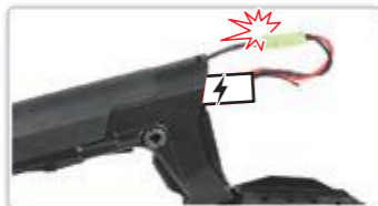
Connect battery until it clicks into place.
