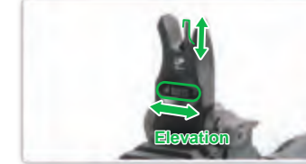
Elevation knob (up / down adjustment).
