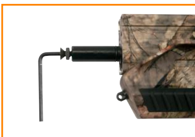
Tighten clamp screw with clockwise 1/4 rotation
