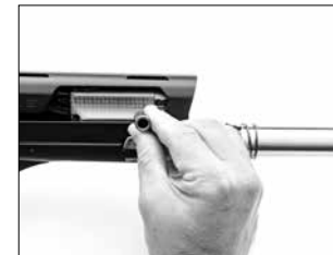
Pull outward to remove the bolt handle.
