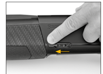
Push the Magazine Cut-Off forward to unblock the magazine.
