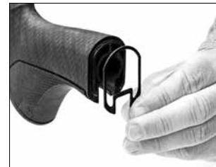
Install the shim between the stock and receiver.
