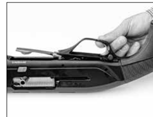
Lift the trigger group from the receiver.
