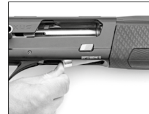
Insert the shell into the bottom of the receiver and push it fully forward into the magazine.
