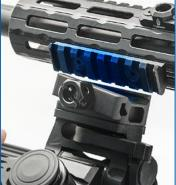
2. Loosen the side locking plate nut by turning it counterclockwise. Loosen it enough for the mounting interface to seat evenly onto your firearm's MIL-STD-1913 Picatinny rail and with its squared recoil stop fitting into the rail slot.
