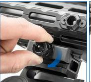
3. Retighten the side locking plate nut by turning it clockwise until snug or to 50in-lb using a torque wrench equipped with a 5/8" socket.
