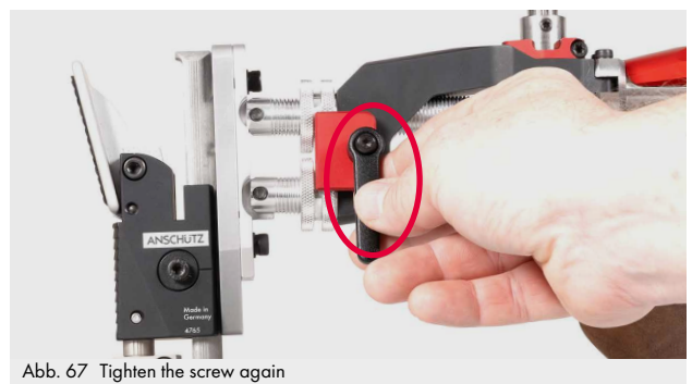
Abb. 67 Tighten the screw again
