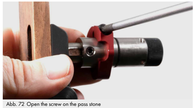
Abb. 72 Open the screw on the pass stone
