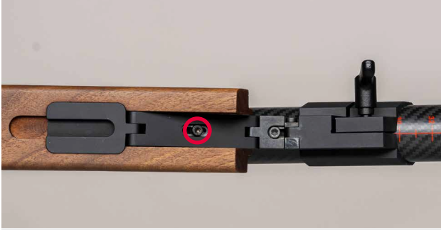
Abb. 86 Loosen the screw
