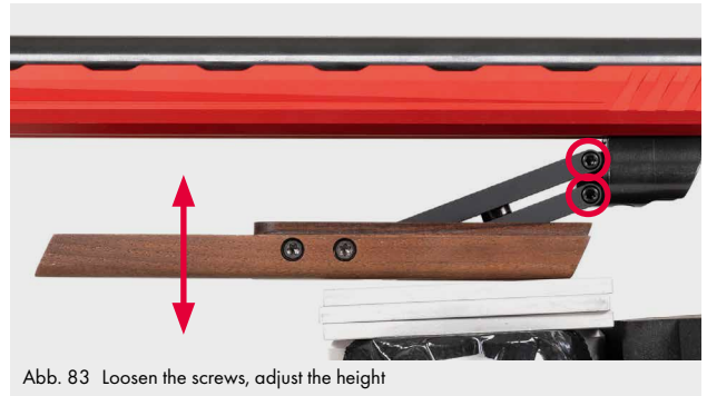
Abb. 83 Loosen the screws, adjust the height
