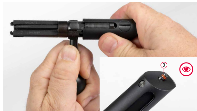
Abb. 9 Bolt cocked - indicator pin visible
