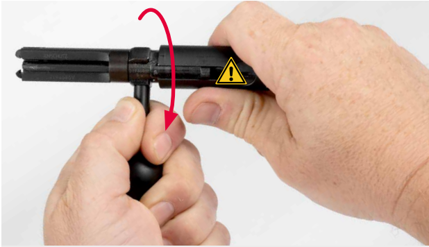
Abb. 15 Uncocking the bolt
