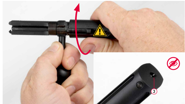
Abb. 8 Bolt uncocked - indicator pin not visible
