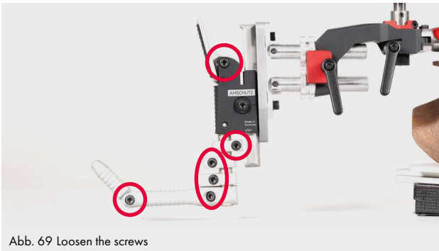
Abb. 69 Loosen the screws
