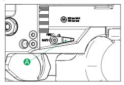
Move the safety lever (A) to the «SAFE» mark position to lock the weapon.
