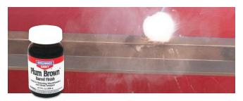
When the ideal temperature of 275°F has been obtained, apply Plum Brown Barrel Finish with a saturated swab in long even strokes. The rich plum brown color will appear immediately. (\*Read Carmichel's Tip below).
