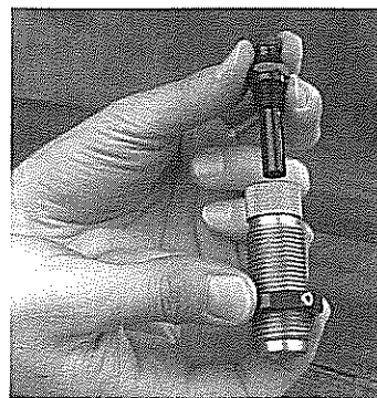
Some seater dies in our 3-die sets use a "through-the-top" style seater plug as shown in this photo. This style allows for easy cleaning.
