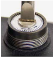
J-3. Use a flat head screwdriver to adjust the windage and elevation.
