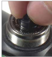
J-5. Apply gentle force on the plastic tab and dial the knob.
