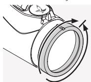
First, turn the diopter adjustment ring fully to the left (counter-clockwise) and then to the right until the reticle is in sharp focus. The adjustment range depends on the individual model. You can find more information in the enclosed technical data sheet.
