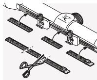
The cover provided can be used to protect the exposed areas of the rail. You can cut it to the required size and press it into the rail using your fingers.
