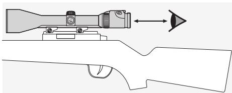
Set the eye relief correctly for a scope mounted on a firearm (see the technical data sheet for the measurements).
