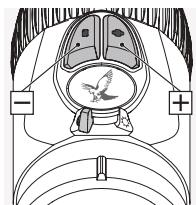
You can now adjust the brightness in the mode you have selected using the  $+$ / $-$  buttons. To reach the ideal level of brightness quickly, you can press and hold one of the buttons (long pulse). To make precision adjustments, press either of the buttons once (single pulse).
