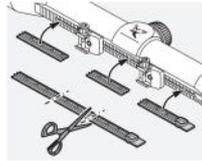
The cover provided can be used to protect the exposed areas of the rail. You can cut it to the required size and press it into the rail using your fingers.
