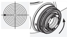
Turn the outer knurled ring on the side turret in the direction of R (counter-clockwise).
