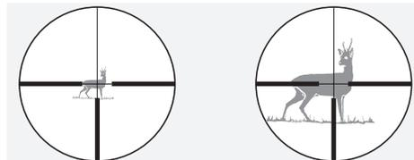
Even at high magnification, only a thin area of the target is covered. The reticle can only be used for estimating the distance to a limited extent.
