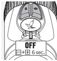
You can deactivate the SWAROLIGHT function by turning the OFF/DAY/NIGHT switch to the central position and pressing the +/- buttons at the same time for 6 seconds. The light will flash twice to confirm
