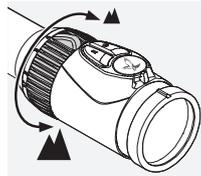
Turn the magnification adjustment ring through up to 180° to obtain the required magnification. The adjustment is continuous. The scale on the adjustment ring makes it easy to see the setting. The soft ribbed cover of the adjustment ring has a small protrusion to make orientation easier. Depending on the model the magnification adjustment ring provides a catch at 1x magnification (CLICKONE), which makes you aware that you are entering the VIEWPLUS area.
