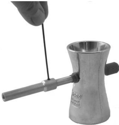
Photo 4 Secure extension tube set screw
