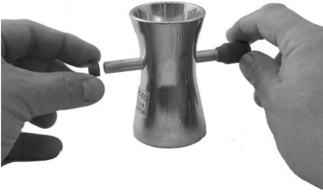
Photo 3 Insert tube and install retaining ring
