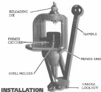
Solidly mount the Reloader Special-5 Press to a sturdy table or workbench with two 3/8" bolts of sufficient length to penetrate the press base and bench. We do not recommend using "C" clamps to mount the press to the reloading bench. Bench bench. Remove the handle nut from the handle and install the threaded portion through the toggle block as shown.
