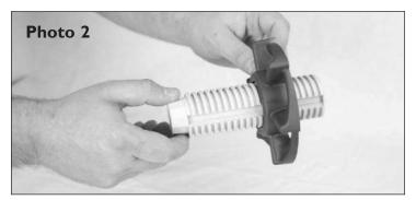
2. Turn the thumbscrew counterclockwise and far enough to install the ram and assembly into the base. Fully install the ram and wheel assembly, allowing the wheel to rest into the base. Secure the ram and wheel assembly into position using the thumbscrew. See **Photo 3**.
