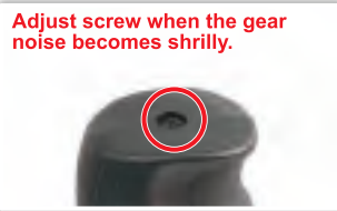
Use a screwdriver to adjust the screw at the bottom of the grip.
