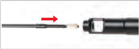
2.Insert the cleaning rod into the inner barrel, turning the rod as you insert. Repeat same steps until barrel is clean.
