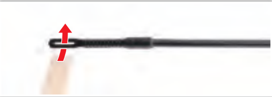
1.Place a few drops of silicone oil or teflon oil on the cleaning cloth and wind the rod around.
