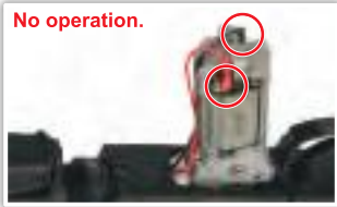
Check the wire set contact on the motor.
