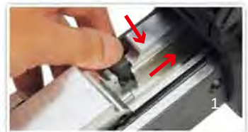
Turn the adjustment nub counter clockwise to raise the bi-pod. Turn clockwise to lower.
