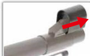
Front sight adjustment Remove the front sight hood.
