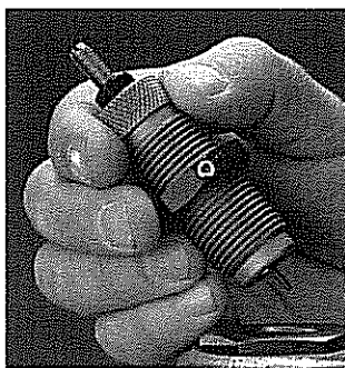
Screw the sizer die into the reloading press.
