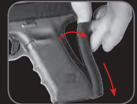
Remove GLOCK Backstrap, if it is mounted.
