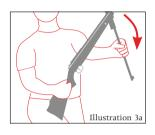
Grasp the barrel near the muzzle end, just behind the muzzle. Pull downward and to the rear until it comes to a solid stop. You will hear a click indicating that the spring piston has been locked into position (see Illustration 3a). Do not let go of the barrel.
