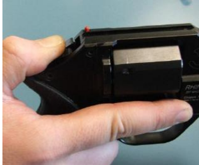
Figure 1 : Cocking the external hammer
