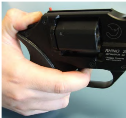
Figure 3: Releasing the external hammer
