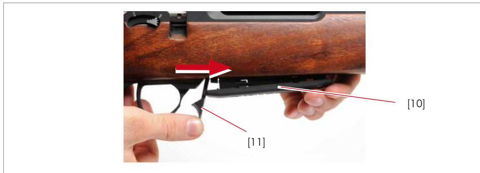
Fig.2 Unlocking the magazine
