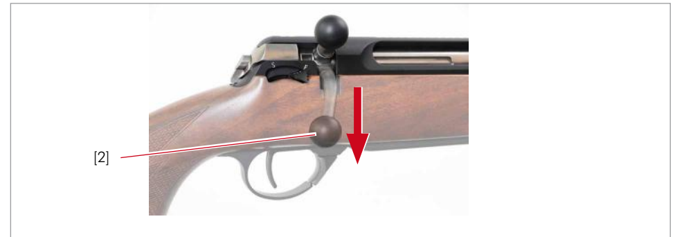
Fig. 16 Pivoting the bolt handle downwards
